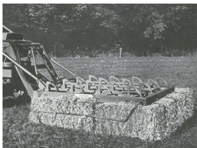
Fig 8 an example of a Flat 8 baler, picking up 8 small bales together
